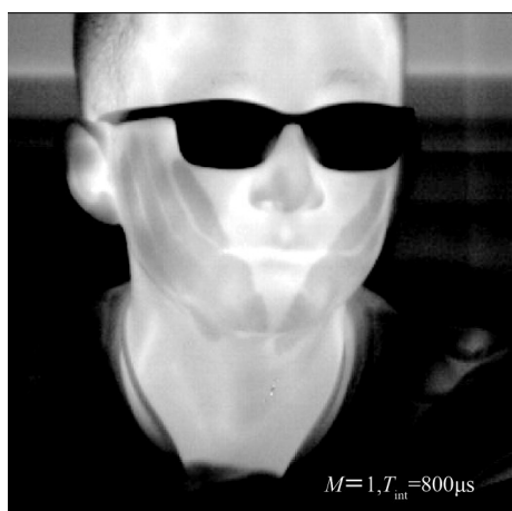
图 14 碲镉汞 APD 焦平面在 -50 mV 反偏下成像演示 Fig. 14 Imaging demonstration of a HgCdTe APD focal plane under V_{\text{bias}} = -50 \text{ mV}
