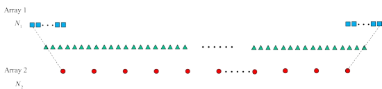
Fig. 3 Diagram of MIMO linear array configuration adopted by the traditional MIMO mechanism 图 3 传统 MIMO 体制线性天线阵列配置示意图
