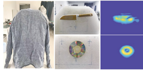
Fig. 15 Imaging test of the targets under clothes
