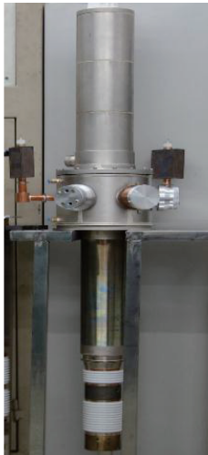
Fig. 8 Photo of the designed gyrotron with quasi-optical mode converter
