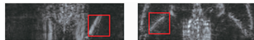
Fig. 5 When a concealed object is placed with its background, there are clear contrasts between the object (knife) and the Interference (arm) 图5 当把隐匿物品放置于背景中时, 隐匿物品(刀)和干扰(胳膊)的对比就很清晰了
