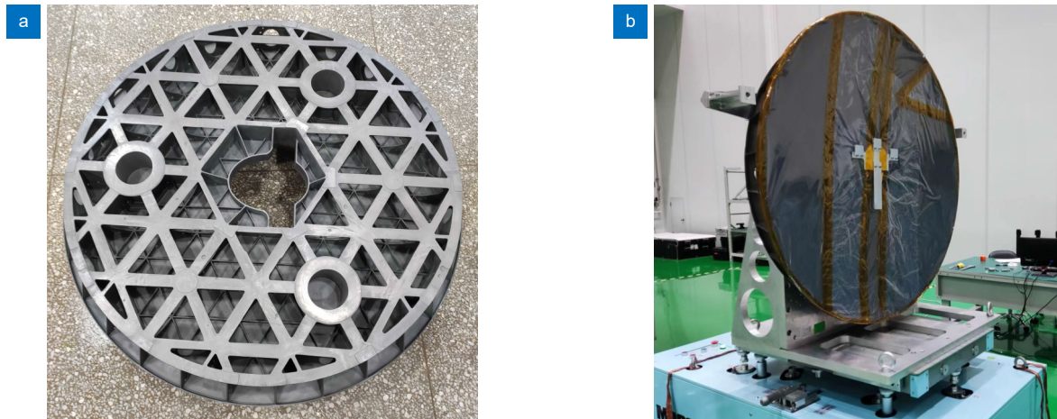
图 9 主镜镜坯制备结果。(a) 镜坯实物; (b) 质心位置测试 Fig. 9 Manufacturing results of the primary mirror blank. (a) Mirror blank; (b) Centroid position test
