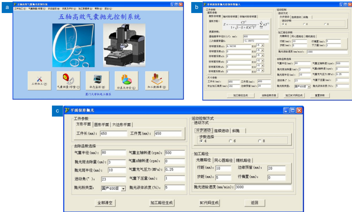
图 24 五轴高效气囊抛光控制系统。(a) 控制软件主界面; (b) 平面保形抛光; (c) 非球面修正抛光 Fig. 24 5 axis high efficiency bonnet polishing control system. (a) Main interface of the control software; (b) Plane conformal polishing; (c) Aspheric correction polishing
