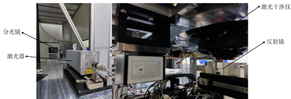
图 6 双频激光干涉仪实物图 Fig. 6 Object picture of the dual-frequency laser interferometer
