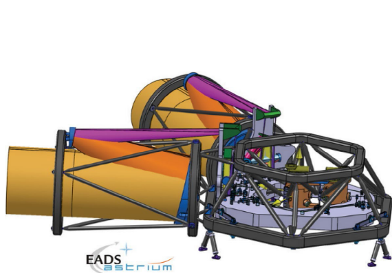
图 14 离轴视场内指向望远镜构型 [43] Fig. 14 Configuration of telescopes with in-field pointing [43]
