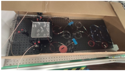
图 11 干涉测量实验装置 Fig. 11 Interferometric measurement experimental setup
