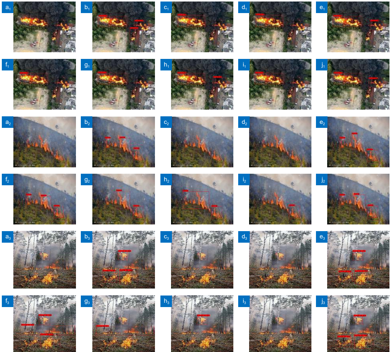
图 9 D-fire 数据集比较实验检测结果。(a) Images; (b) Ours; (c) EFDNet; (d) Y-Edge; (e) M-YOLO; (f) Fire-YOLO; (g) YOLOX-Tiny; (h) PicoDet; (i) PP-YOLOE; (j) YOLOv7;
