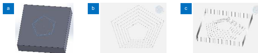
Example of algorithm validation. (a) Schematic diagram of damage contour construction; (b) Yin mold processing point constructed by algorithm; (c) Yang mold processing point constructed by algorithm
