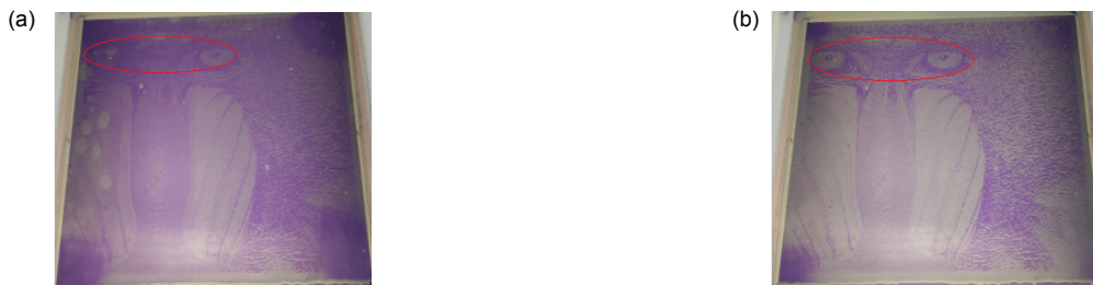
图 15 两种不同驱动波形下的显示对比图。(a) 9 阶灰度图；(b) 15 阶灰度图 Fig. 15 Visual contrast between two kinds of driving waveform. (a) 9 grayscales image; (b) 15 grayscales image
