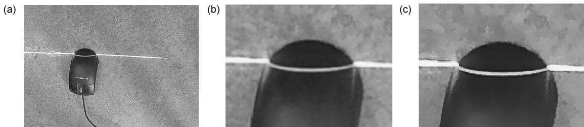
图 1 激光条纹原图及处理图像。(a) 激光条纹原始图; (b) 高斯滤波处理结果图; (c) 双边滤波处理结果图 Fig. 1 Original laser stripe image and processing image. (a) Original laser stripe image; (b) Result of bilateral filter; (c) Result of Gaussian filter
