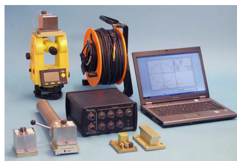
图7 SCHILL公司的308型舰船轴线检测系统 Fig. 7 Model 308 ship axis inspection system of SCHILL
