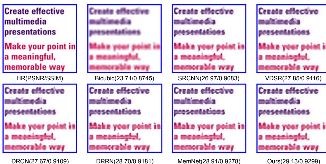
图 8 Set14 数据集中的“ppt3”图片 3×重建 Fig. 8 “ppt3” from Urban with an upscaling factor of 3×
