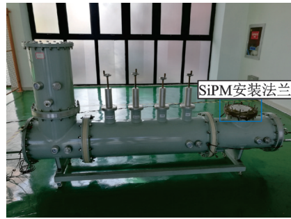
图 8 SiPM 现场验证试验 Fig.8 SiPM field verification test
