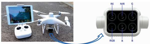
图1 大疆精灵4 RTK多光谱无人机及其成像系统 Fig.1 DJI Phantom 4 RTK multispectral UAV and its imaging system
