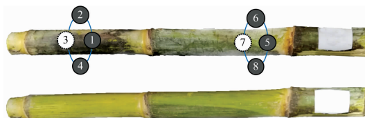
图2 去蜡前后的甘蔗样本及透射光谱采集位点示意图 Fig. 2 The sugarcane samples before and after wax removal and the sketch of transmittance measurement positions
