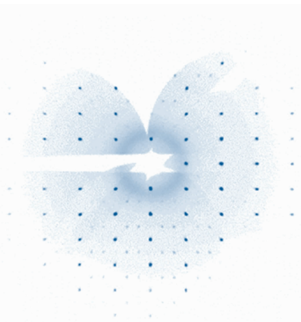
图 1 \text{Sm}(\text{CO}_3)\text{OH} 单晶 X 射线衍射点阵图 Fig. 1 \text{Sm}(\text{CO}_3)\text{OH} single crystal X-ray diffraction lattice
