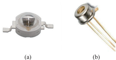
图 1 光源和传感器。(a) 红外 LED 光源;(b) 钢镓砷光电二极管 Fig.1 Light sources and sensors. (a) Infrared LED light source; (b) InGaAs photodiode
