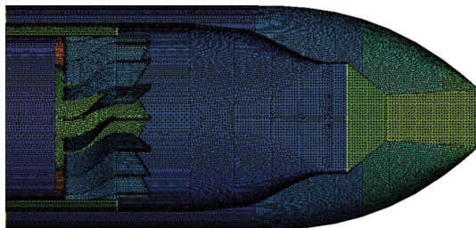
(b) 组合模型壁面网格 (b) Grid of combined model wall
