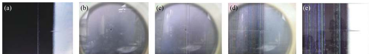
图 5 带镜头的 CMOS 在 1064 nm 激光能量增加时的损伤效果图。(a) 0.4 ms 激光对 CMOS 损伤效果图; (b)~(e) 10 ns 激光对 CMOS 损伤效果图 Fig.5 Damage effect picture of the CMOS with lens under increasing 1064 nm laser energy. (a) Damage effect of 0.4 ms laser on CMOS; (b)-(e) Damage effect of 10 ns laser on CMOS
