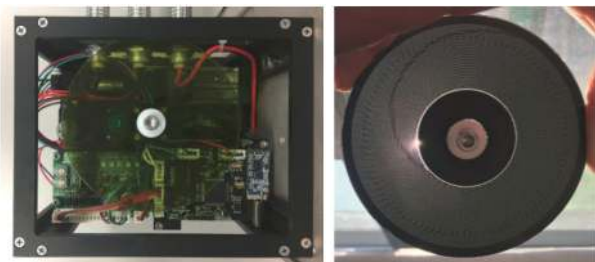
(a) 装配完整的推力器 (b) 被烧蚀的靶盘 (a) Complete thruster assembled (b) Ablated target disk
