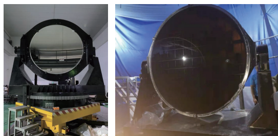
(a) \Phi 2.7 m 球面镜 (b) \Phi 2 m 平面镜 (a) Spherical mirror of \Phi 2.7 m (b) Plane mirror of \Phi 2 m
