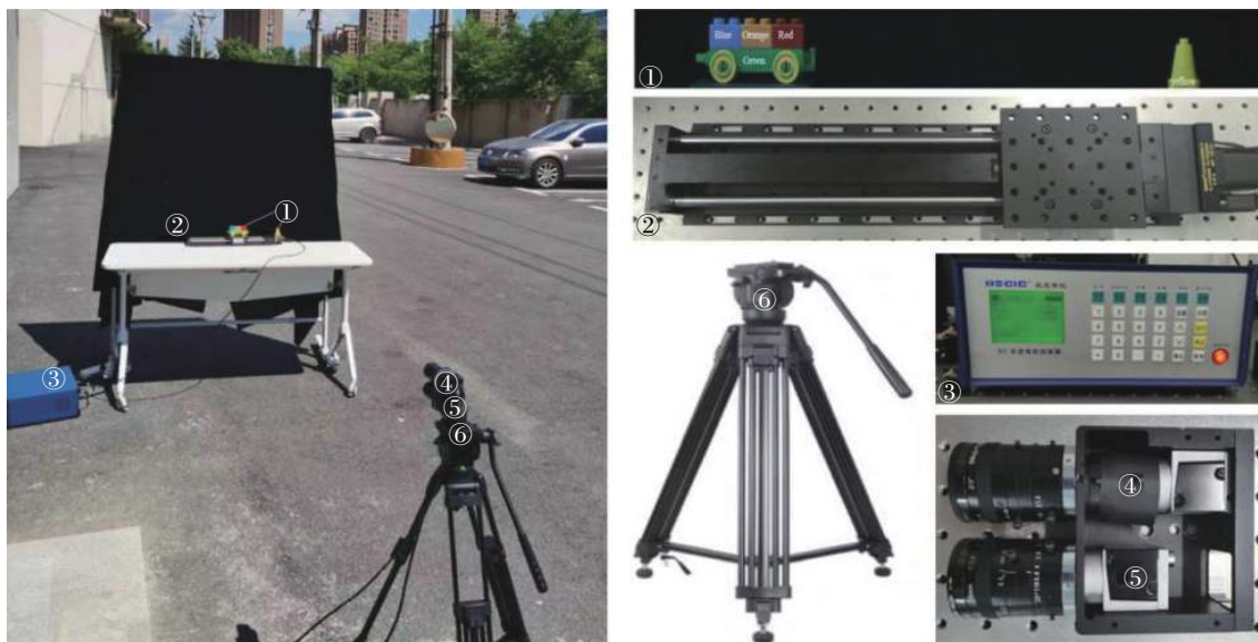
图 3 外场实验装置图。①目标物体; ② SC100 型步进电机; ③ SC 步进电机控制器; ④ GISC 相机; ⑤ RGB 相机; ⑥ KINGJOY VT-2500 三脚架 Fig.3 Diagram of the experimental setup in the field. ① Target object; ② SC100 stepping motor; ③ SC stepping motor controller; ④ GISC camera; ⑤ RGB camera; ⑥ KINGJOY VT-2500 tripod
