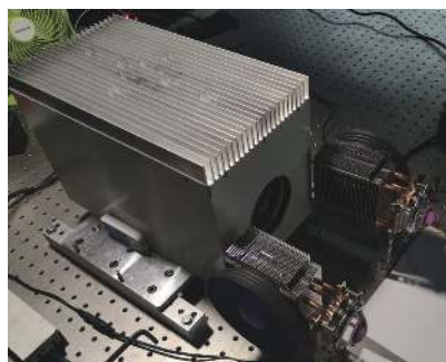
(b) 相机热控系统实物 (b) Camera thermal control system physical object
