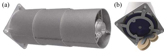
图 15 (a) 展开状态下的镜筒; (b) 安装在主镜后面的弹簧马达 Fig.15 (a) Deployable barrel in deployed configuration; (b) Spring motor mounted below primary mirror
