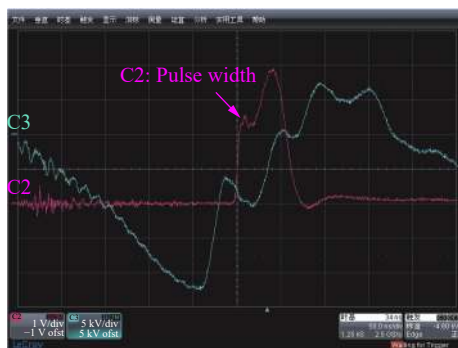
(a) 阻抗不匹配 (a) Impedance mismatch
