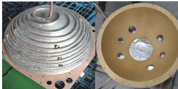
图 1 第一版红外积分球辐射源的盘管挂锡和真空镀金实物图 Fig.1 The first edition practical picture of coil tin hanging and vacuum gold-plating of infrared integrating sphere radiation source
