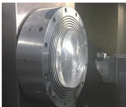
Fig.12 Ultra-precision machining of Fresnel lens
