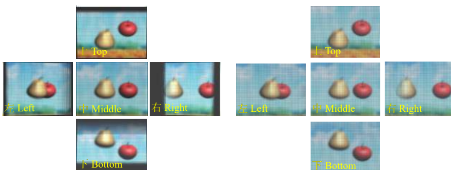
(b) 传统两步拍摄法的重建 3D 图像 (b) Reconstructed 3D images of conventional two-step pickup method (c) 无黑边的两步拍摄法的重建 3D 图像 (c) Reconstructed 3D images of proposed two-step pickup method without black zone
