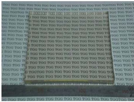
图 3 日本神岛化学制备的超过 10 \times 10 cm 尺寸的 TGG 陶瓷 [42] Fig.3 TGG ceramic with a size over 10 \text{ cm} \times 10 \text{ cm} prepared by Konoshima Chemical, Japan [42]
