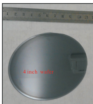
(c) 4 in 碲镉汞分子束外延材料 (c) 4 in HgCdTe MBE material
