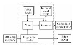
Fig.5 Architecture of the CHT module
