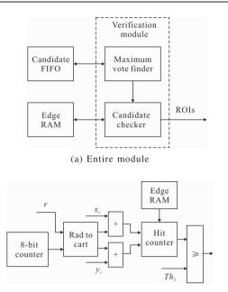
(b) Candidate checker submodule Fig.7 Architecture of the verification module
