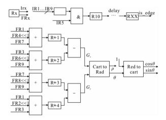
Fig.4 Pipeline for calculating the edge flag and gradient direction
