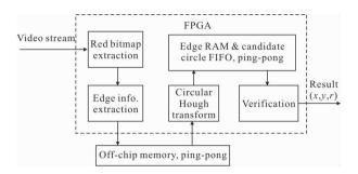
Fig.3 Block diagram of the proposed architecture
