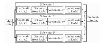
Fig.6 Architecture of the voter submodule
