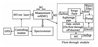
Fig.2 Block diagram of the laser fluorometer instrument
