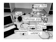
(a) Instrument schematic diagram
