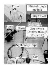
(b) Flow-through measurements schematic diagram Fig.1 Instrument configured for the discrete and flow-through measurements
