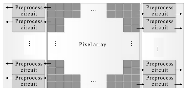
Fig.1 Pixel array and the preprocess circuit
