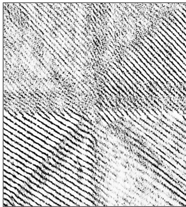
Fig.5 Interference pattern of RPB and polarized Gaussian beam
