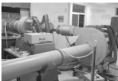
图 4 试验内外涵气流系统 Fig.4 Primary and bypass flow systems
