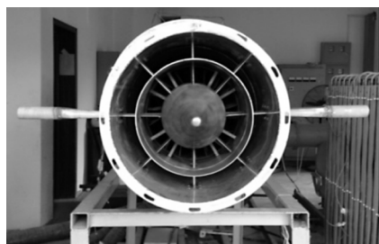
图 3 喷管前部部件图 Fig.3 Front view of nozzle
