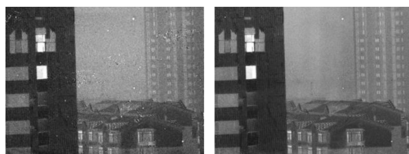
(g) 校正前场景 4 偏振度图像 (h) 校正后场景 4 偏振度图像 (g) Polarization image of scene 4 before NUC (h) Polarization image of scene 4 after NUC
