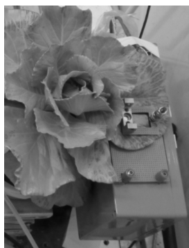
Fig.2 A view of the experimental plant and the leaf clamping system on the laser speckle imaging apparatus placed inside the chamber
