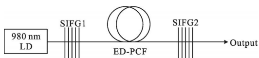
Fig.1 Experiment devices of the dual-wavelength Er 3+ -doped PCF laser based on SIFGs
