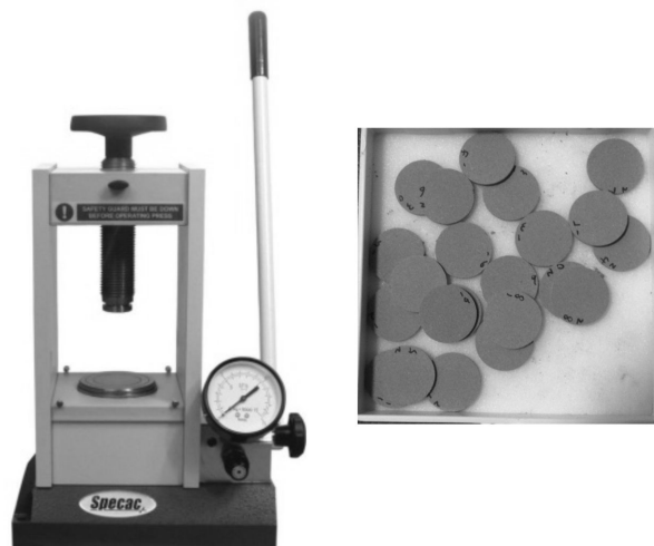
(a) Pressed-slice making machine
