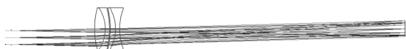
(d) 焦距 400 mm,工作距 350 mm,光阑直径 \Phi 17 mm,入瞳距 86 mm (d) Focus 400 mm, working distance 350 mm, diameter of entrance pupil \Phi 17 mm, distance of entrance pupil 86 mm
