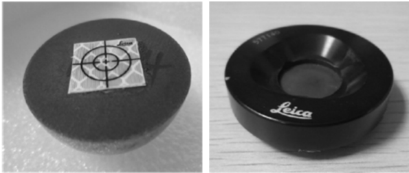
(a) 标定半球 (b) 磁性基座 (a) Calibration hemisphere (b) Target holder
