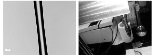
(a) Tapered fibers observed under the microscope (b) Tapered fibers physical figure
