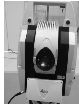
图 1 激光跟踪仪 Fig.1 Laser tracker
