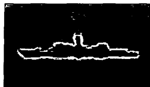
图 3 加噪后统计法对军舰图的边缘检测结果 Fig.3 Edge detection result of adding noise warship image by statistic method
