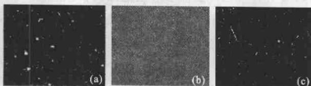
(a) 第 30 帧图像 (b) 第 30 帧图像预处理后的结果 (c) 目标轨迹 (a) The 30th frame (b) Preprocessed result of the 30th frame (c) Target track of the 30th frame
