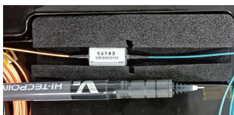
Fig. 5 Fabricated integrated optical field sensor for MV/m pulsed electric-field
